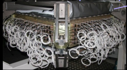
电磁量能器 Electromagnetic Calorimeter (ECAL)
