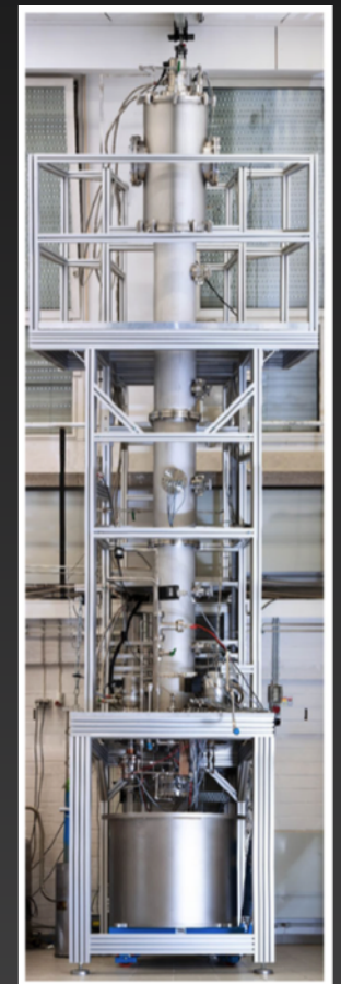
Krypton distillation column
