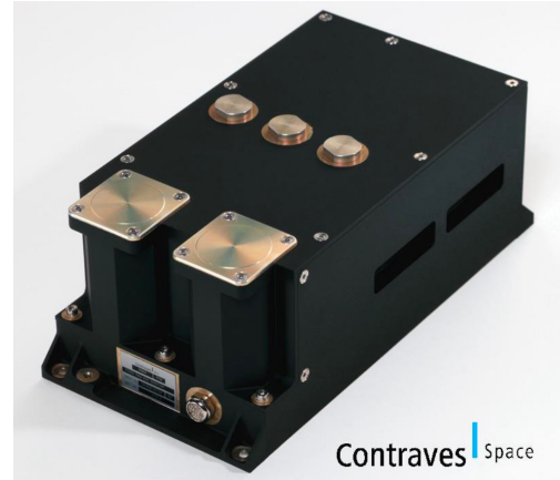
SREM (Standard Radiation Environment Monitor) Dimension: 9.5 \times 12 \times 22 \text{ cm}^3 Mass: 2.64 kg Consumption: 2.5 W Dynamic range: electrons from 0.3 MeV to 6 MeV and protons from 8 to 300 MeV Mission: Integral, Rosseta, Planck, etc
