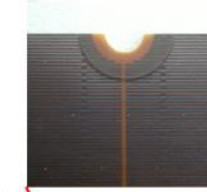
Central upper hole for layer interconnection. Readout strips routed around the hole. Central separation of resistive pattern.
