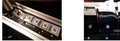
Fig. 4. *Left*: 6 Tiles on motorized sled. On the leftmost the cylinder containing the source is visible. *Right*: UV LED fiber system under each tile.
