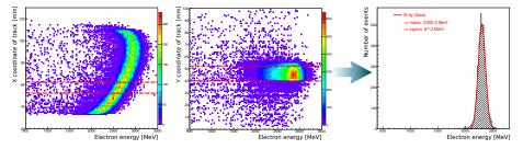
•  $\Delta_E/E$  for electron beam with trigger area of  $\pm 5$  mm horizontally and  $\pm 5$  mm vertically relative to the central trajectory.
