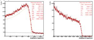
• The calibration results of energy scale (left) and energy resolution (middle) for the BGO-calorimeter. Comparison of energy resolution of calorimeters (right).
