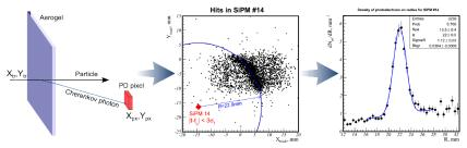
• Many pixels can be combined to improve accuracy and align the tracking system with the PD pixels.
