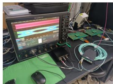
Uplink Eye Diagram tests
