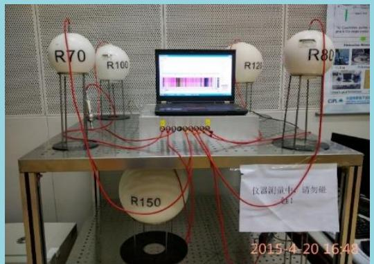
9 spheres neutron spectrometer
