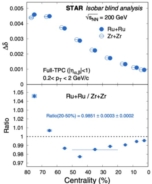
FIG. 7.  $\Delta\delta$  measured for Ru + Ru and Zr + Zr collisions at  $\sqrt{s_{NN}} = 200 \text{ GeV}$  (upper panel) and the ratio of Ru + Ru to Zr + Zr (lower panel). The centrality bins are shifted horizontally for clarity. The border-less horizontal bands denote the statistical uncertainties. The horizontal bands with the dashed border represent the systematic uncertainties.
