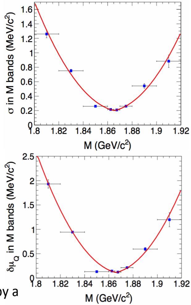
Correlation btw.  $\sigma_{\text{effective}}$  and  $M$ ,  $(\mu_G - \mu_{\text{Stu}})$  and  $M$  by a 2-order polynomial function of  $|M - \mu|$
