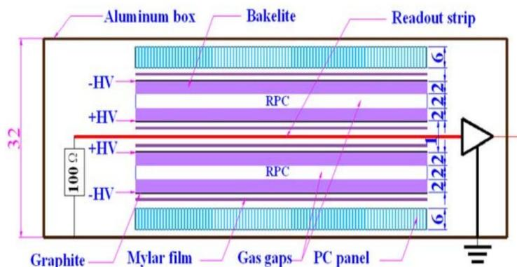
Figure 2.5 The cutaway drawing of a RPC superlayer module.
