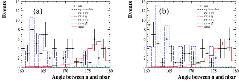
**Figure B.4** Angle between  $n$  and  $\bar{n}$  after selection for (a) 2.2324 GeV and (b) 2.40 GeV.
