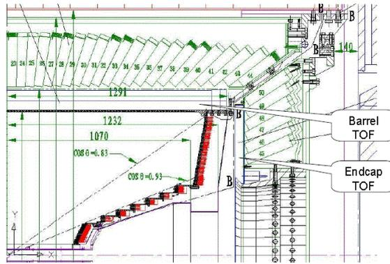
**Figure 2.3** Schematic structure of TOF at BESIII.
