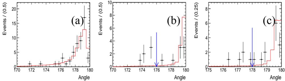
**Figure 4.28** The distributions of opening angle between  $\Lambda$  and  $\bar{\Lambda}$  in center-of-mass system at (a) 2.40 GeV, (b) 2.80 GeV and (c) 3.08 GeV.
