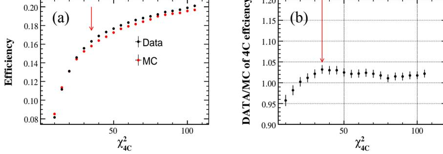
**Figure 5.16** (a) Kinematic fit efficiency between data and MC from control sample. (b) The difference of the efficiency between data and MC.
