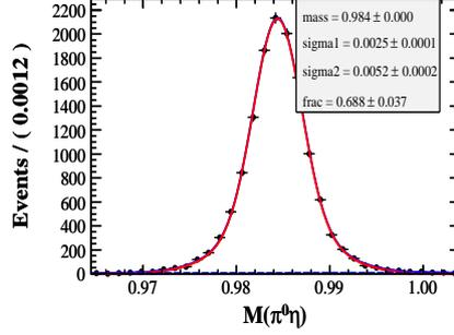
**Figure 5.9** Invariant mass spectrum of  $\pi^0\eta$  on signal MC with 0-width  $a_0(980)$ , fitted with Double-Gaussian function.
