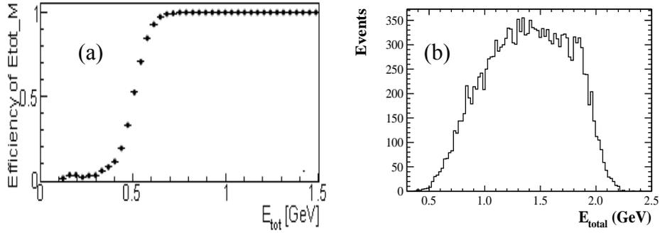
**Figure 4.25** (a)Efficiency of the medium energy threshold versus total EMC energy. (b) Total EMC energy in signal MC process  $e^+e^- \rightarrow \Lambda\bar{\Lambda} \rightarrow \Lambda\bar{n}\pi^0$ .
