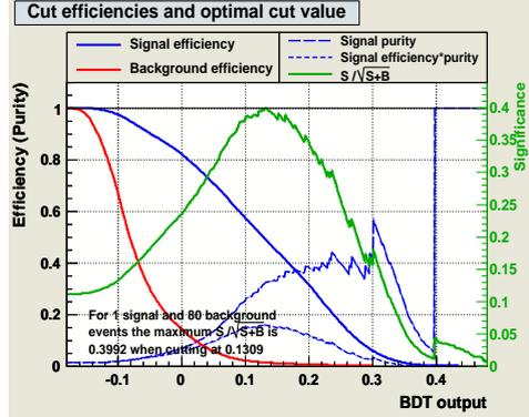
**Figure 4.16** The cut efficiencies with different output classifier applied with 100 signal and 500 background events assumption for BDT classifier.
