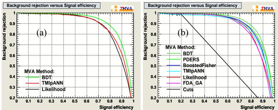
Figure 4.14 Background rejection versus signal efficiency for different classifier outputs.
