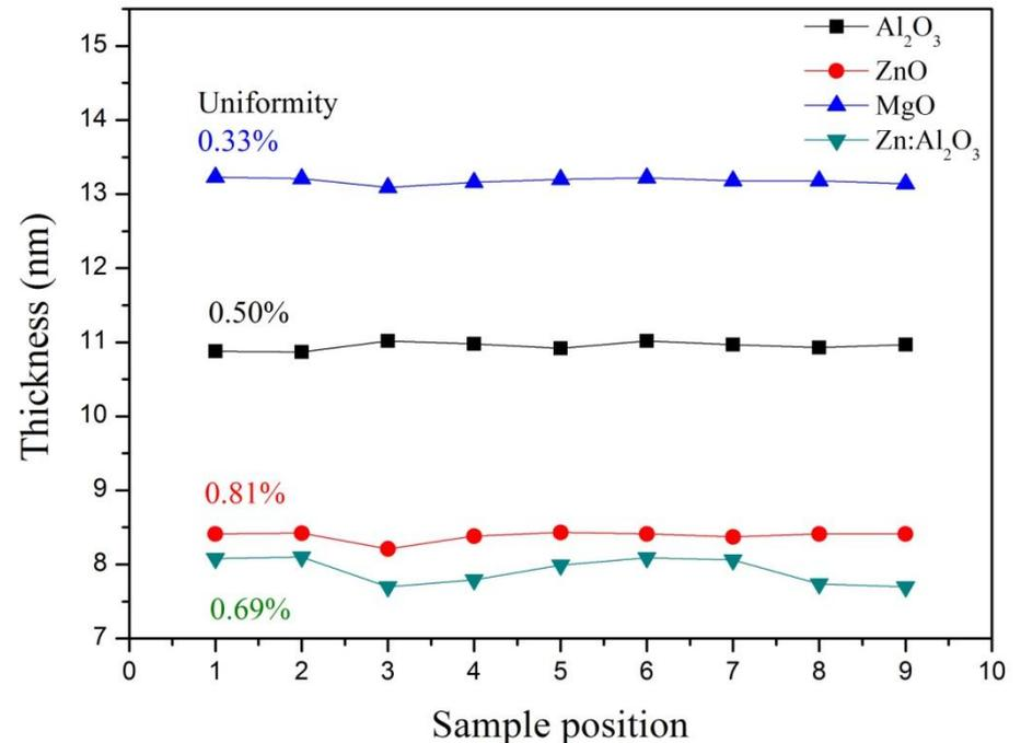
The thickness of MgO,  $\text{Al}_2\text{O}_3$ , ZnO, and AZO deposited on 4" silicon substrate by ALD are 13.18 nm, 10.95 nm, 8.38 nm, and 7.92 nm, thickness uniformity are 0.33% , 0.5% , 0.81% and 0.69%, respectively.
