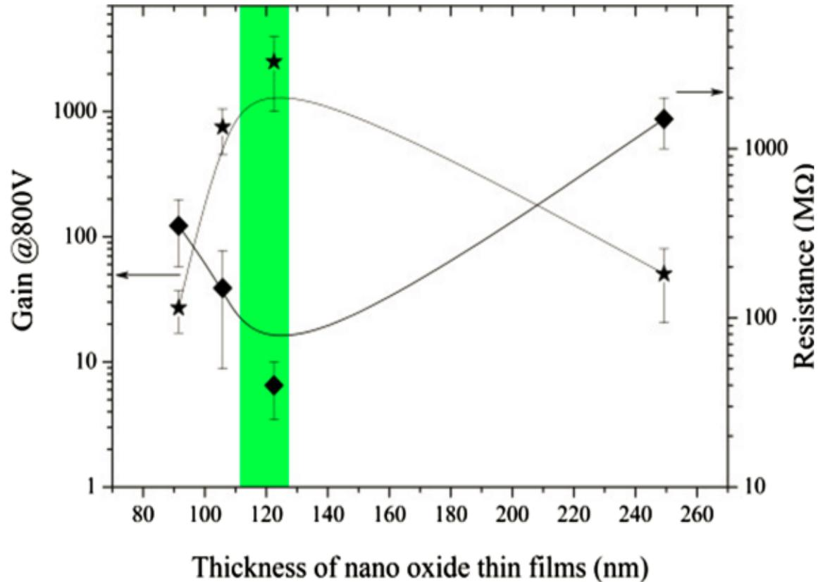
Gain and resistance of ALD-MCP as a function of nano-oxide thin film thickness
