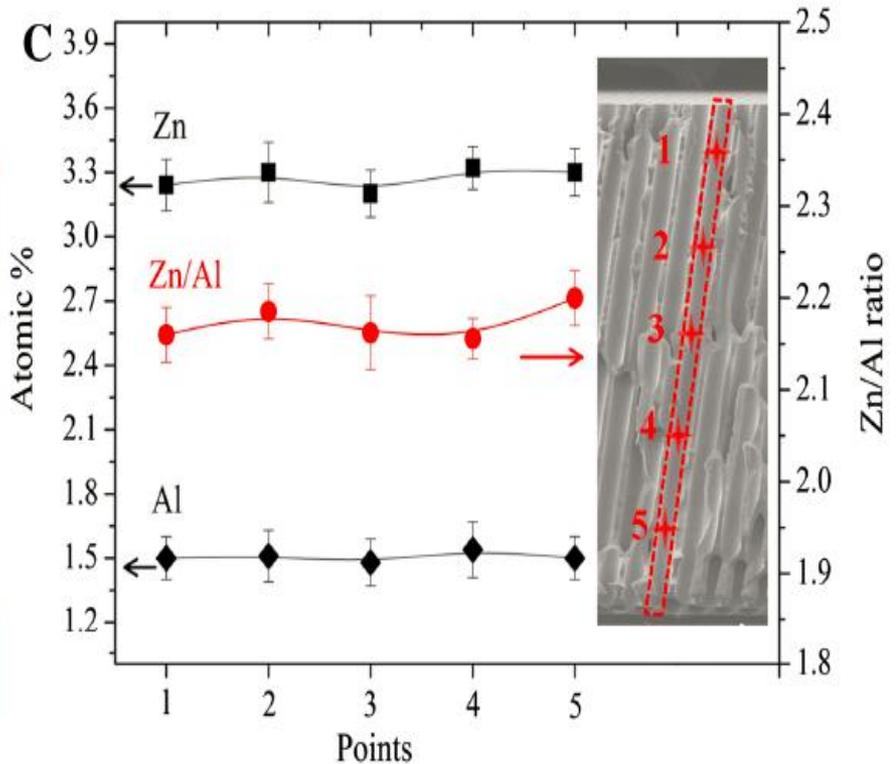
The spectra and elemental composition of cross-sectional bare MCP and ALD-MCP samples
