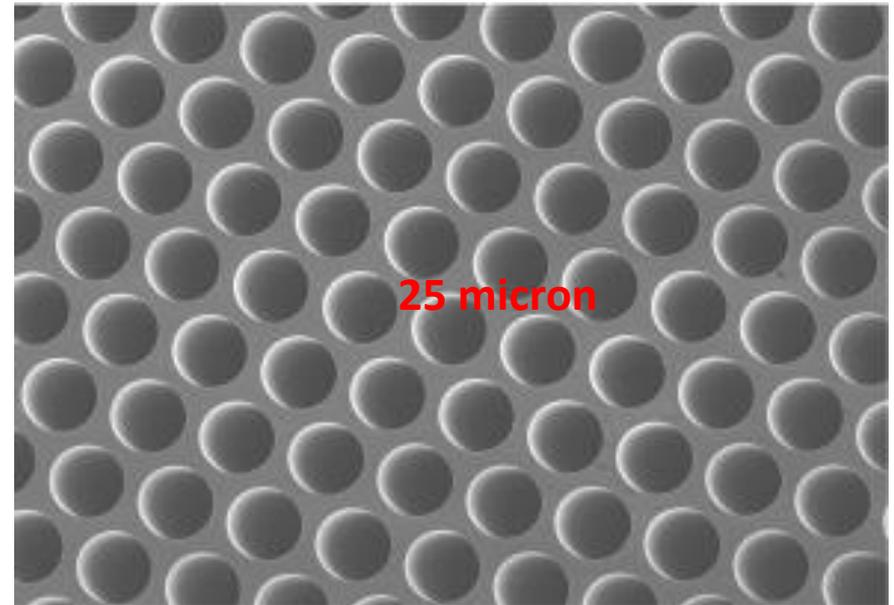
the top-view SEM picture of nano-oxide
