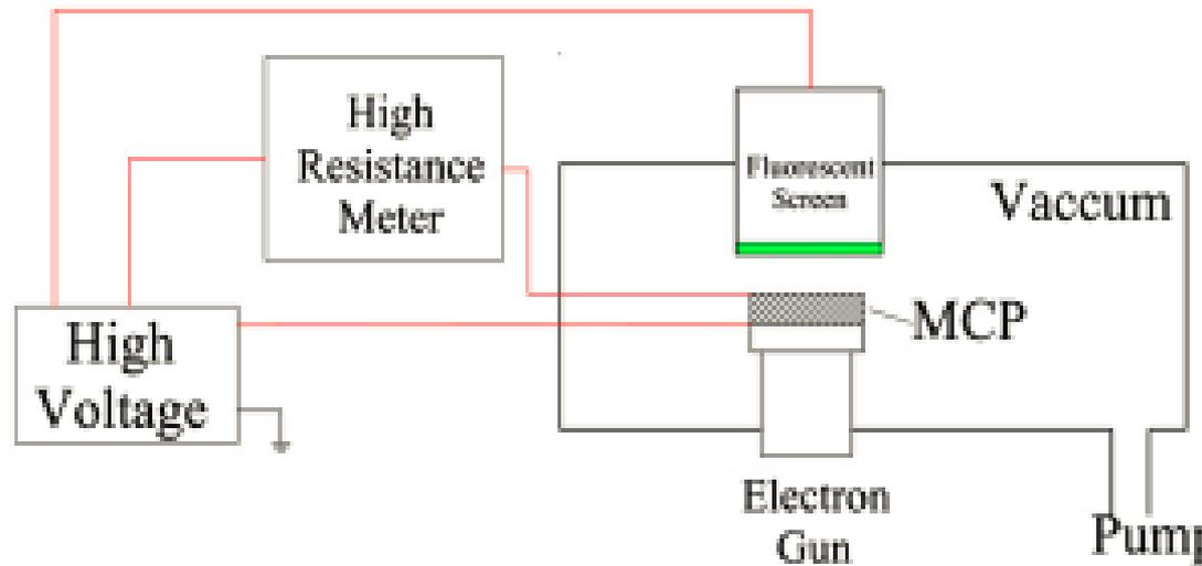
MCP electrical measurement system
