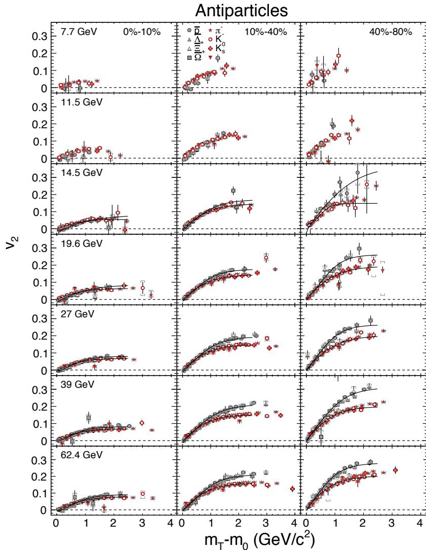
The splitting between baryons and mesons is observed significant for all energies above 14.5 GeV and also at 14.5 GeV for 40%–80%.
