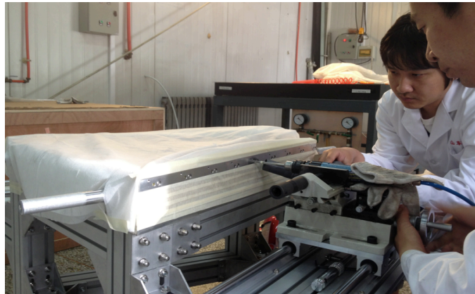
Pining the wire mounts
