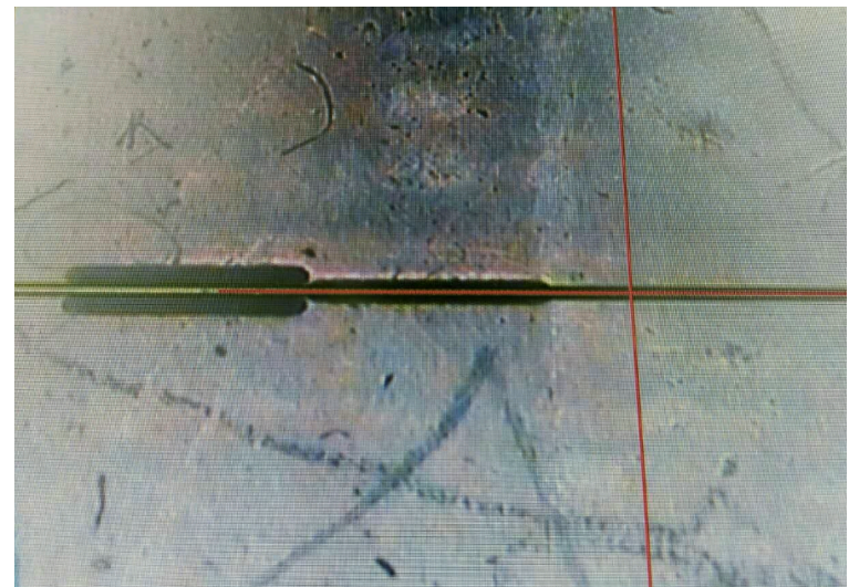
Epoxying anode wire mounts
