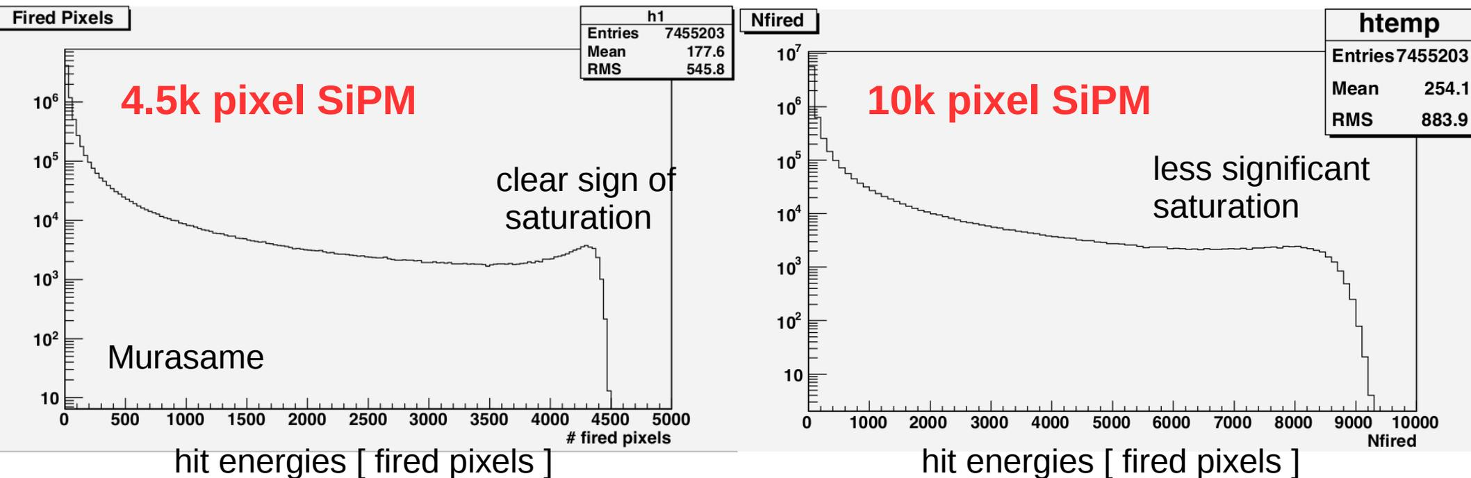
1x1 mm<sup>2</sup> 10k pixel MPPCs available, but difficult to operate with current readout ASIC
