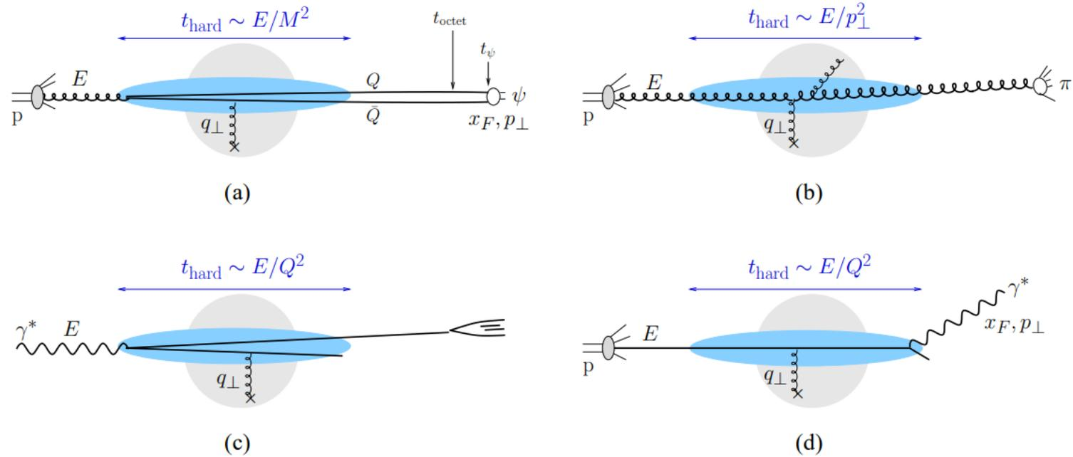
**Figure 1.** Generic processes of (a) heavy-quarkonium hadroproduction (b) light hadron hadroproduction (c) deep inelastic scattering and (d) Drell-Yan production, at large  $E$  in the target nucleus rest frame. The ellipse represents the hard subprocess occurring within the time  $t_{\text{hard}}$ . Cases (a) and (b) are similar to small angle scattering of an asymptotic charge.
