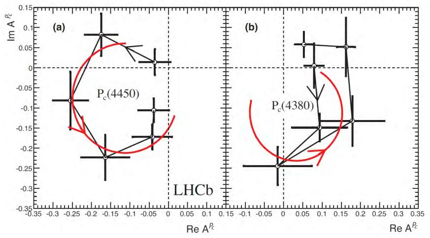
$P_c(4450)$ : predicted, narrow:  $\Gamma=39\pm5\pm19$ , 10 MeV from  $\Sigma_c\bar{D}^*$  threshold perfect Argand plot: a molecule
